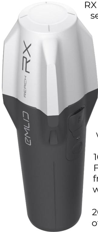
RX is waterproof up to 1.5 m depth. All connectors are completely sealed and protected from water and dust with silicone plugs.
